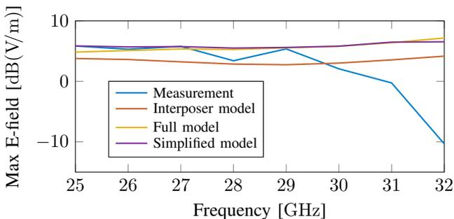
Fig. 9. Maximum electric field value at 3 m for an input power of 1 W for the matched microstrip with right angle.
