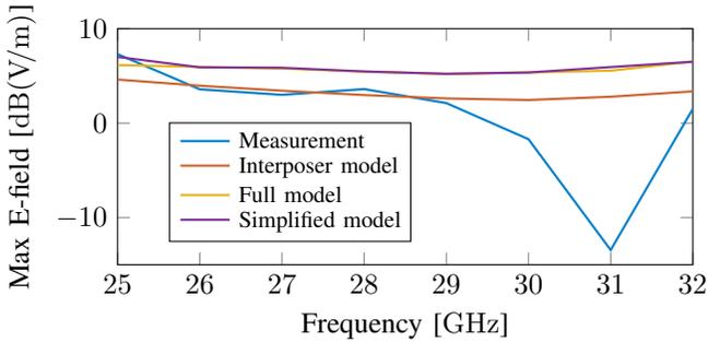
Fig. 8. Maximum electric field value at 3 m for an input power of 1 W for the shorted microstrip with right angle.
