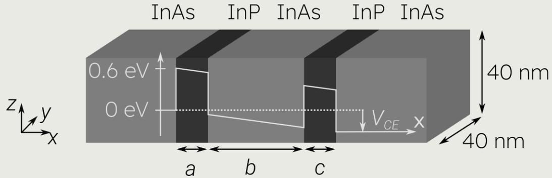
Double barrier structure allows only specific energies to pass.
